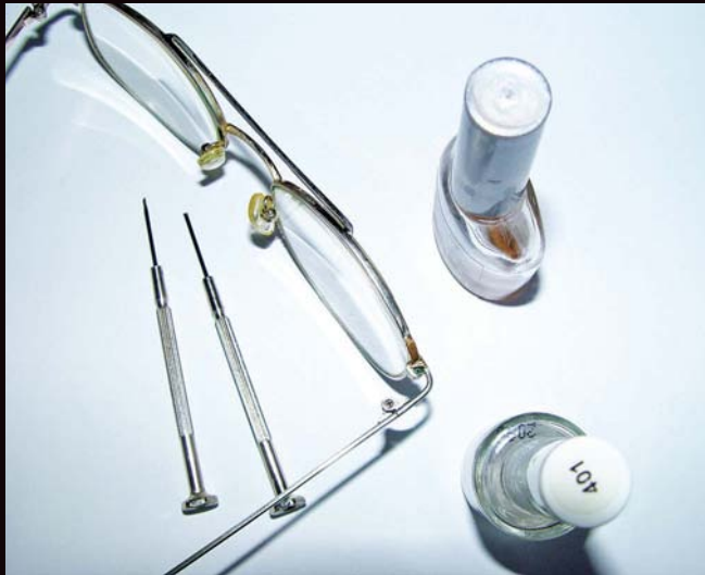
The tiny screws holding the lenses of your eyeglasses in place can sometimes loosen and become lost. An easy way to prevent this is to remove the screws, and place a dab of clear nail polish on the threads prior to screwing them back into place.
