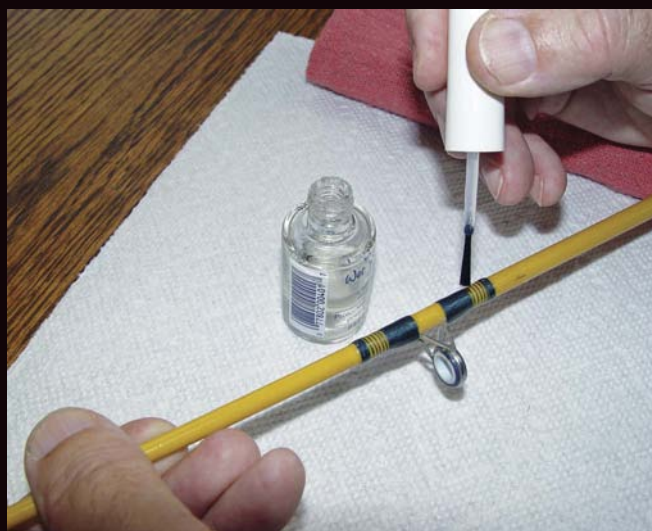
The guide wrapping on fishing poles can eventually start to wear. An application of clear nail polish easily repairs those damaged areas and discourages further unwinding.
