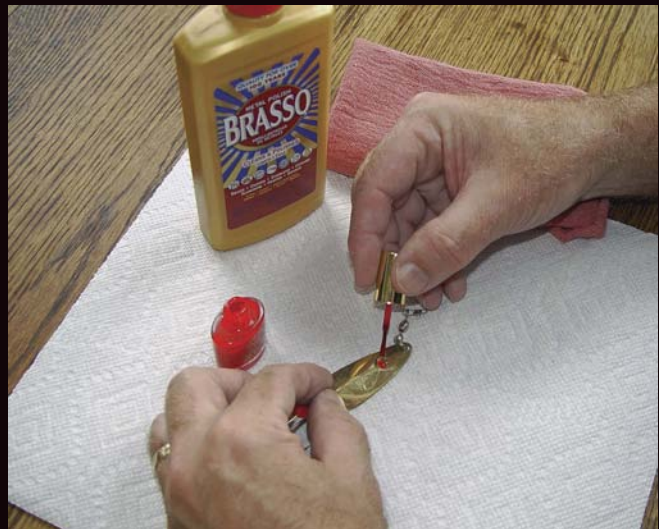
Polishing compounds like Brasso can be used to bring luster back to the bare metal surfaces of fishing lures. After that, applying a protective coat of clear nail polish will help them resist damage and tarnishing.
